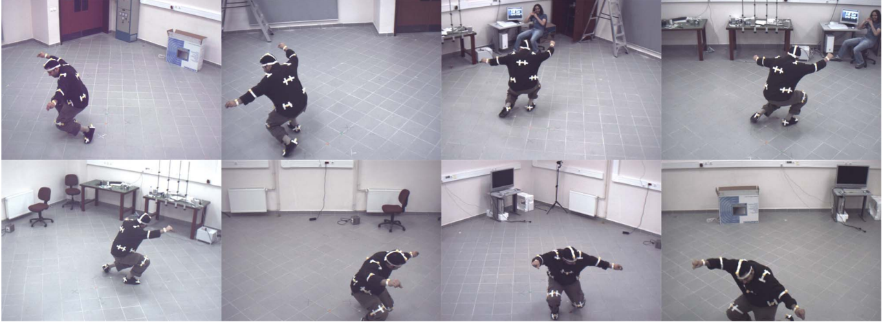
Fig. 1. Dance scene captured by the 8-camera system available at Koç University. Markers are attached at or around the joints of the body.
